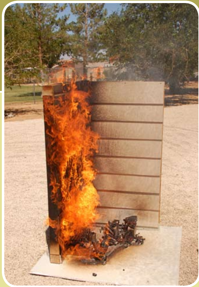
we are looking at vertical flame spread on a combustible siding product. Noncombustible siding is shown on the right hand side of the wall. Both wall sections had the same initial fire exposure.
